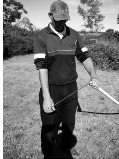
2) Bend a piece of very heavy fencing wire or light steel reinforcing rod so that a 1-metre arm is at right angles to the top of the pipe.
